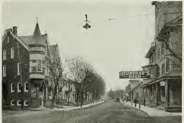
Fig. 3. Day View of Main Street, Sellersville, Pa., showing G-E eye suspension fixture equipped with concentric reflector, prismatic refractor and 250-c.p. 6.6-amp. Mazda lamps
