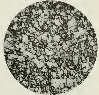
Fig. 4b. Iron-Cobalt,  $Fe_2Co$ , No. 3 Co01, Melted in Vacuo. Annealed. 50 diam.
