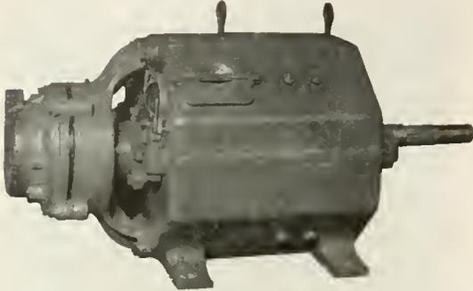
Fig. 11. Boat Crane Motor
