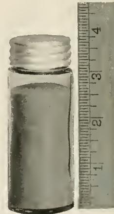
Fig. 4. Sand shown in Vial Represents One Per Cent of Sand by Weight in 12 Lb. of Gear Lubricant
