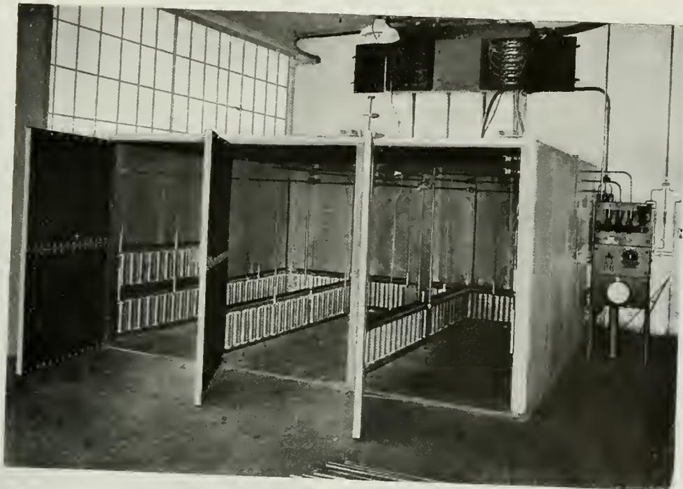
Fig. 1. A View of an Electrically Heated Japan Baking Oven and its Controlling Equipment
