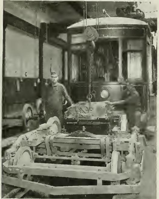
Fig. 3. Removing a 65-H.P. Box Frame Motor from the Truck. This operation takes fifteen minutes to perform
