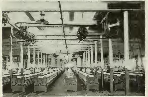
Fig. 11. Typical Group Drive in Ring Spinning Room
