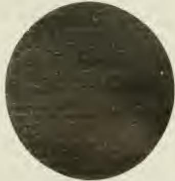
Fig. 5. Photograph of Bottom Surface of Casting at place where piece was cut out. Note that no imperfections are visible at the surface
