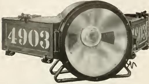
Fig. 5. The Standard Type of Locomotive Headlight for the 6-volt, 108-watt, Focus-type Lamp
