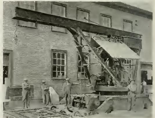
Fig. 8. Electric Locomotive Crane especially designed for delivering blocks to sawing beds at mills
