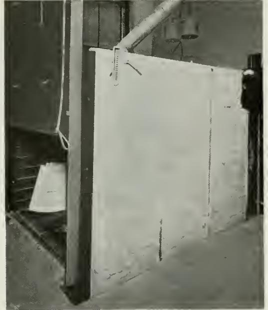
Fig. 5. An Electrically Heated Drying Oven
