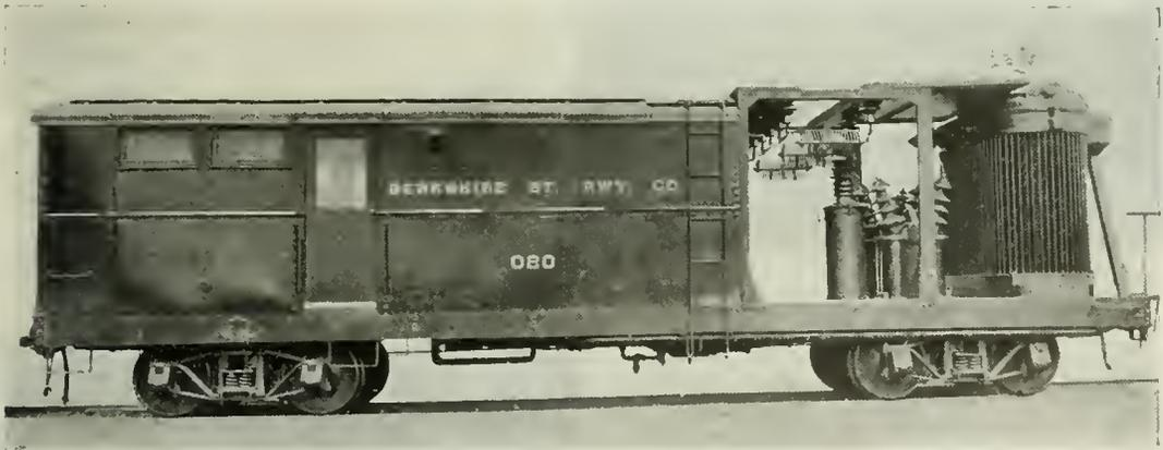
Fig. 1. Side View of the Semi-outdoor Portable Substation
