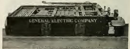
Fig. 14. Combination Storage Battery and Trolley Type Mine Locomotive with Platform Removed to Show Internal Arrangement
