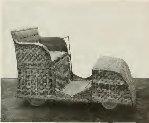
Fig. 1. Electriquette with Split Rattan Body
