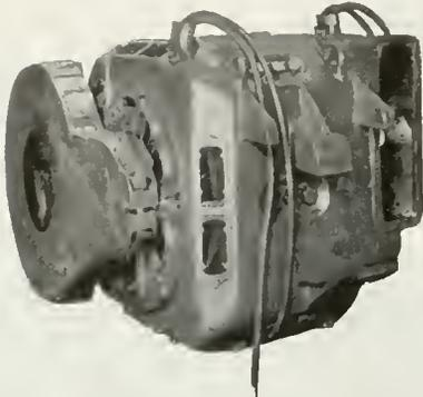
Fig. 8. One of the Eight, 430-h.p., 3000-volt Motors Used for Driving a C., M & St. P. Locomotive
