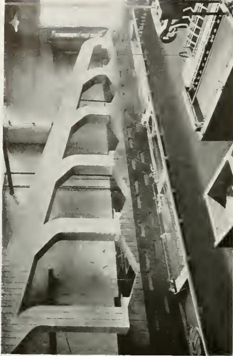
Fig. 4. Portion of Electroplating Room showing Cleaning Tanks, Ventilating Hood, Water Filter and Water Still
