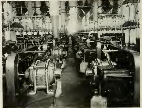
Fig. 13. Motors Direct Connected to Spinning Frames. Erlanger Cotton Mills, Lexington, N. C.
