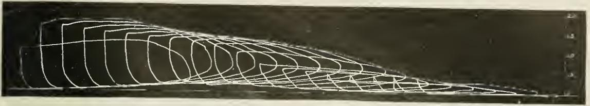
Fig. 2. Continuous Indicator Diagram of Twin Simple Hoist Engine
