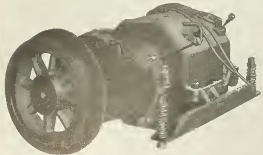
Figs. 2 and 3. HM-803 Mining Locomotive Motor Mounted on Axle
