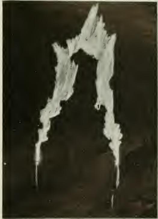
Fig. 3. An Instantaneous Photograph of a 353,000-Volt Arc Produced from a 300,000-Volt Testing Transformer by Conversion Between Terminals 43 Inches Apart. Total Length of Arc about 20 Feet
