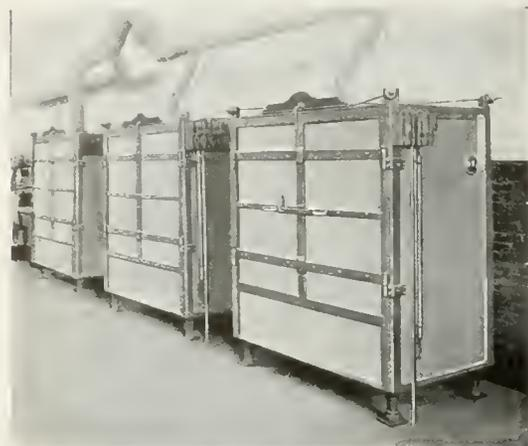
Fig. 3. A Set of Electrically Heated Drying and Baking Ovens
