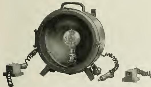
Fig. 8. Incandescent Headlight Designed for Use on Interurban Cars
