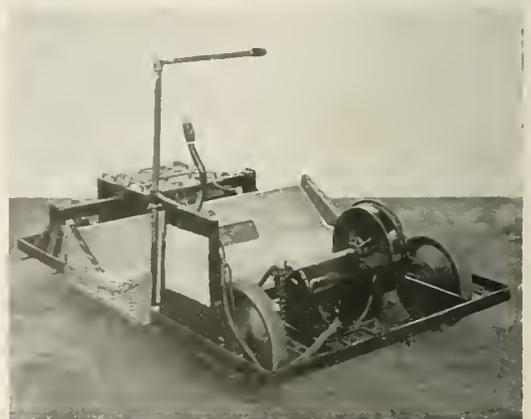
Figs. 2 and 3. Front and Back Views of Electriquette Chassis
