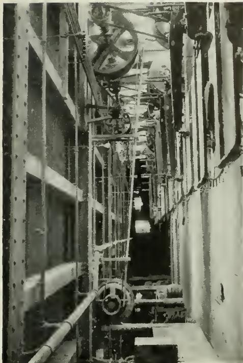
Fig. 56. 50-h.p., Form L, 220-volt Induction Motor Driving 33 Staking Machines in Tannery
