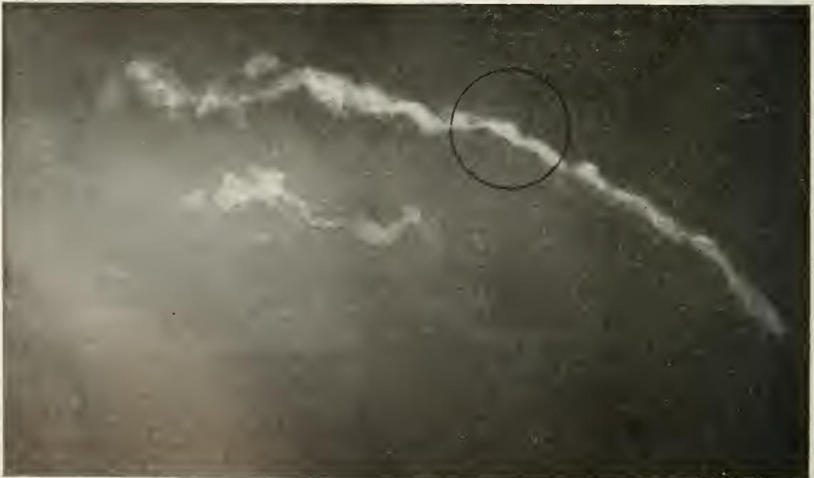
Fig. 1. Radiograph of a Steel Casting showing Flaw within Casting. The circle shows where a piece was later punched out
