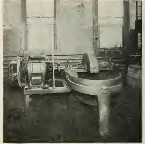
Fig. 46. 20-h.p., 1200-r.p.m., 220-volt, Form K Motor, Direct Connected to Meat Cutter with 40-in. Bowl, 200 Pounds Capacity
