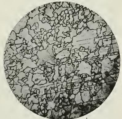
Fig. 5b. Iron-Cobalt,  $Fe_2Co$ , No. 3 Co02, Melted in Vacuo. Annealed. 50 diam.
