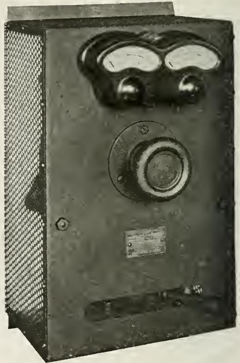
Fig. 9. The Control Panel Used with an A-c.—D-c. Compensarc for Two Lamps Alternately
