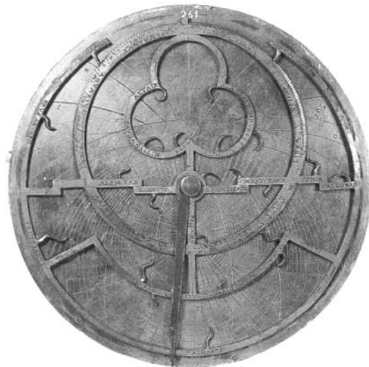
Astrolabes were usually made of brass so that the plates could move smoothly and they could stand up to frequent use either for astronomy or for navigation.
